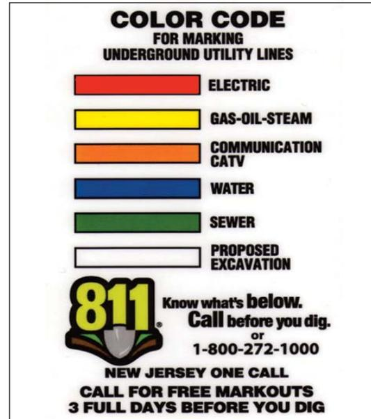
Figure D-12 Utility marking color code.
